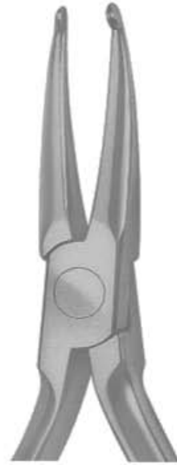
2653 How Plier Tips are 1/8"(3.2mm) diameter
